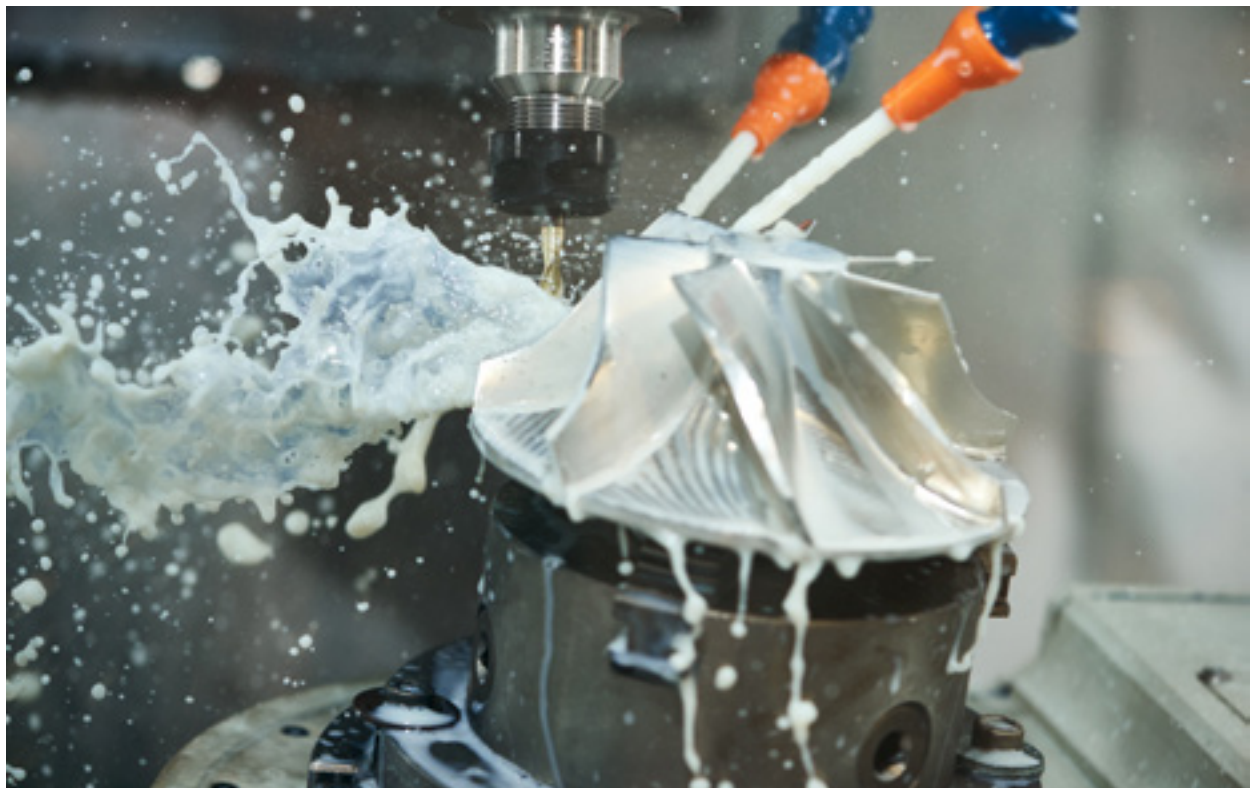
CNC machines can be cheaper than metal 3D printers, but limit geometric freedom
