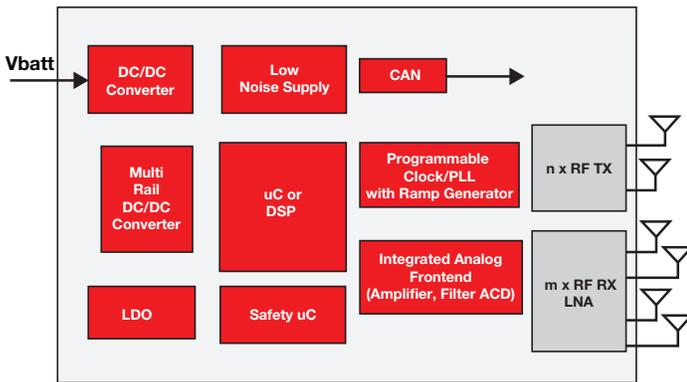
Long-range radar system diagram
