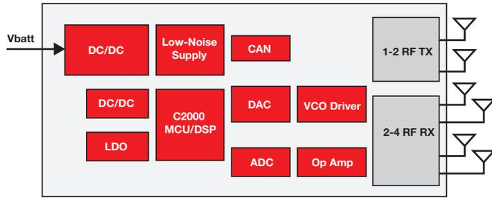
Short- and medium-range radar system diagram
